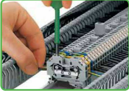
Open the clamping spring using a screwdriver and insert stripped conductor until it hits the stop.
