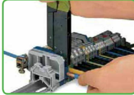
The plunger is placed into the upper operating slot of the side-entry terminal block and the clamp is hooked into the lateral operating slot. The contact is fully opened by pressing the handles together until they engage. Insert stripped conductor until it hits the stop.
