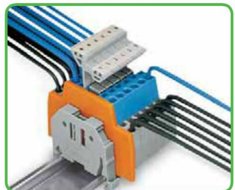
Double deck terminal blocks used as control wire terminals; e.g., magnetic valves. Upper deck commoned.
