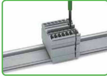
Unlock assembly with screwdriver (3.5 x 0.5 mm / 0.137 x 0.020 in) and remove terminal block via release lever.
