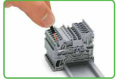
Receptacle terminal block: connection/removal of conductor with screwdriver (3.5 x 0.5 mm / 0.137 x 0.020 in).
