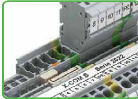
Commoning of receptacle terminal block with staggered jumper. Always push down the jumper until fully inserted!
