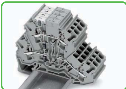
Double-deck diode terminal blocks have been specially developed for custom diode circuits, such as lamp test and collective fault signal circuits. Using LED terminal blocks, monitoring units can be designed, e.g., for control and operating circuits. The terminal blocks provide high-density wiring, while maintaining a width of only 5 mm/0.197 in. Push-in type jumper bars provide additional options for custom circuit design.
