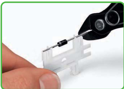
Cutting component to the proper length.
