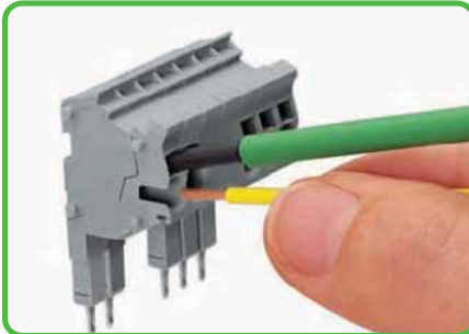
Conductor termination: - Using an operating tool for unferruled, fine-stranded conductors - Push-in connection of solid conductors
