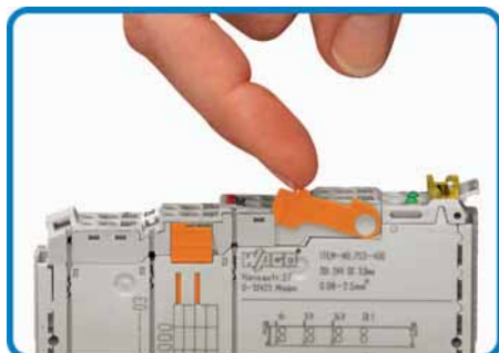
Locate the orange pull-tab on the connector ...
