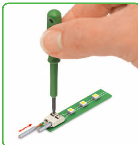
Insert/remove fine-stranded conductors by lightly pressing on push-button (e.g., using a 233-335 operating tool or a ball point pen).
