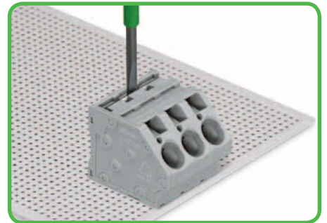
To insert comb-style jumper bar, push it down using a screwdriver until it hits the backstop - 745 Series.
