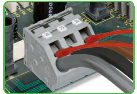
Testing with test plug - 745 Series.
