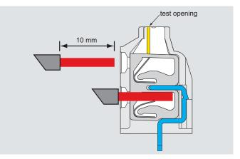
When inserting a flexible conductor with a ferrule and a rigid conductor with a cross section of  $\geq 0.75$  mm<sup>2</sup>, the spring opens automatically. For cross-sectional areas  $\leq 0.75$  mm<sup>2</sup>, it is necessary to open the terminal by pressing the button with a screwdriver.
