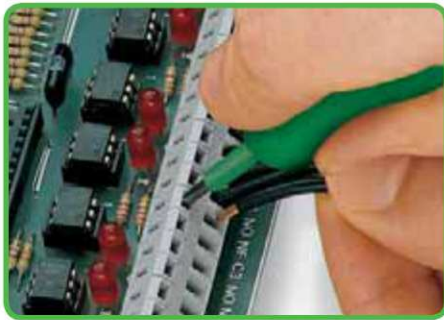
Conductor termination using a screwdriver 3.5 mm / 0.137 in: Wire entry and operation of the clamp are parallel to each other.
