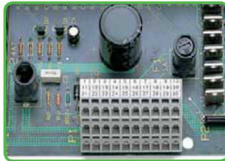
Space-saving triple deck terminal strip.
