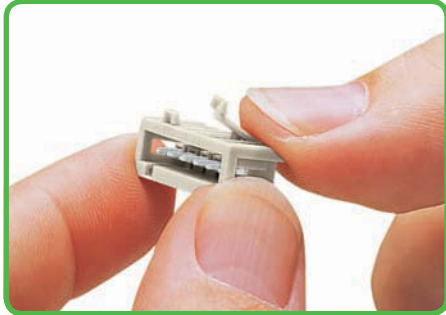
Coding a male header - fitting coding key(s).
