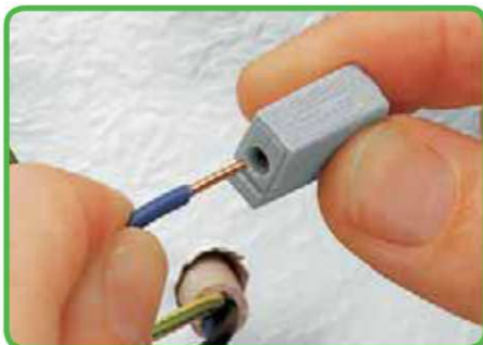
Installation side terminations: Insert stripped solid conductor into entry and push until it hits the stop.
