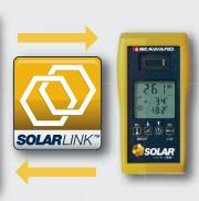
Solarlink™ connectivity enables irradiance to be displayed and for irradiance, module and ambient temperature to be recorded with the PV150 (available separately) in real time as electrical tests are conducted.
