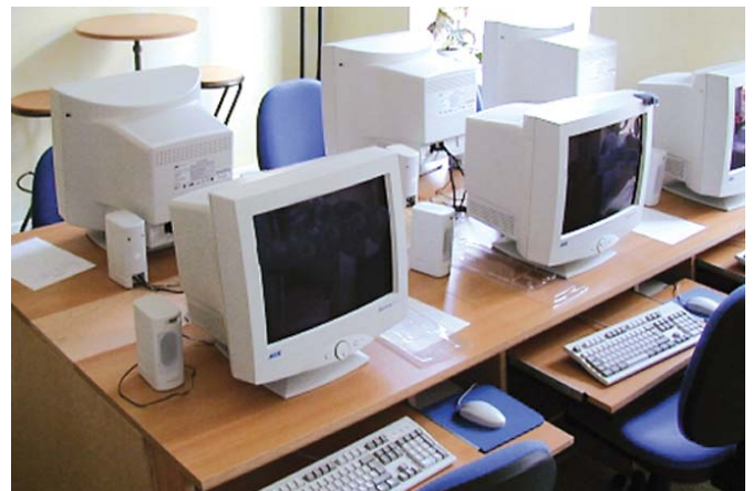
EDP devices can be the cause of harmonics
