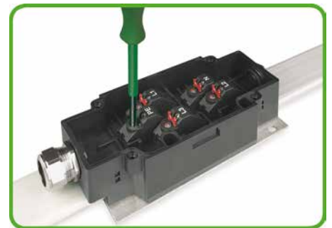
Make contact with the flat cable by tightening the screw until it hits the stop (observe the tightening torque!)
