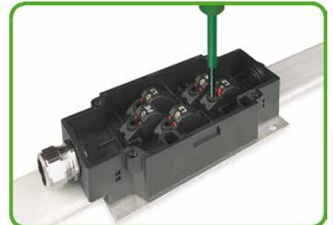
Red contact clips confirm that the contacts are made correctly when they are flush with the terminals.
