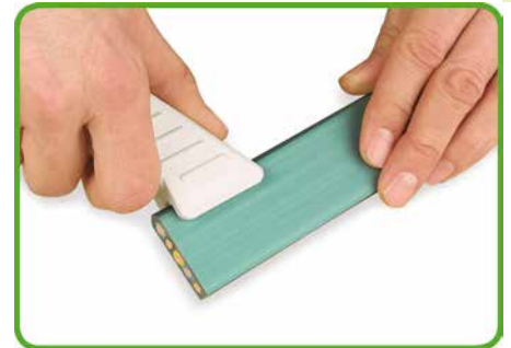
Cut both sides of the outer insulation of the flat cable using a stripping knife (observe 30 mm of cutting length).
