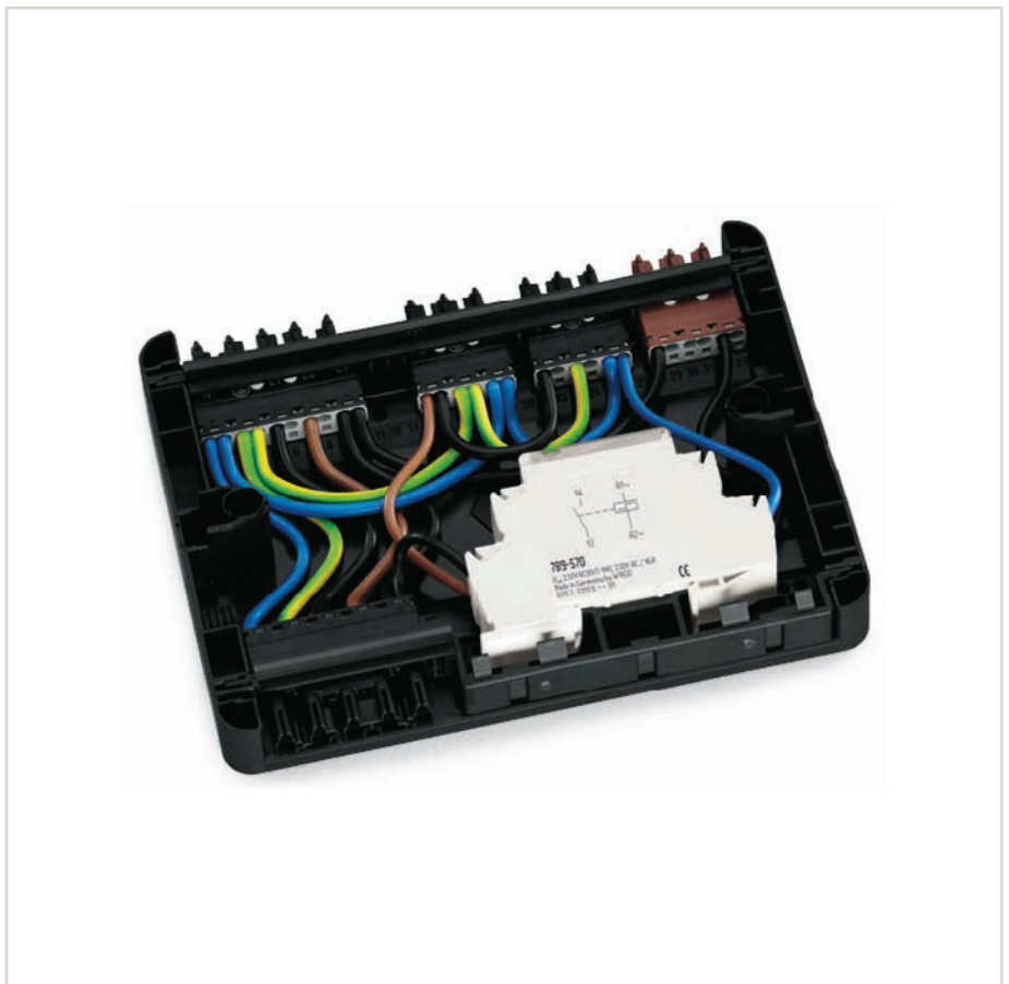
Solid conductors are terminated via push-in termination, while stranded and fine-stranded conductors are inserted using an operating tool.
