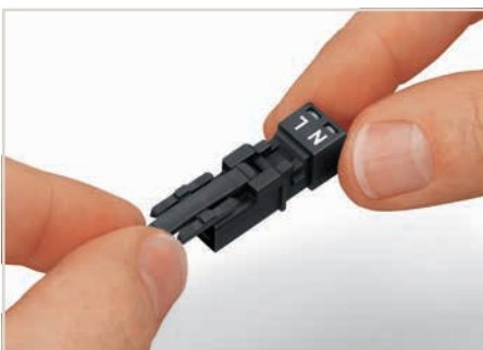
All connectors for mounted installations (snap-in versions, pluggable PCB connectors, distribution connectors) are factory-equipped with locking levers to ensure plugs and sockets are securely locked. Additional locking levers are only required for flying leads (plug/socket).
