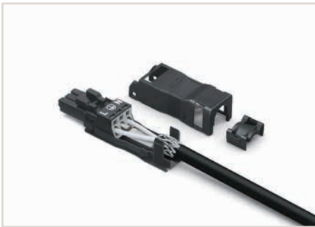
First insert wired connector into strain relief housing, then snap the clamp and cover.
