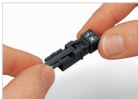
All connectors for mounted installations (snap-in versions, pluggable PCB connectors, distribution connectors) are factory-equipped with locking levers to ensure plugs and sockets are securely locked. Additional locking levers are only required for flying leads (plug/socket).
