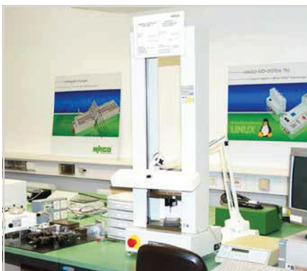
Conductor retention force testing
