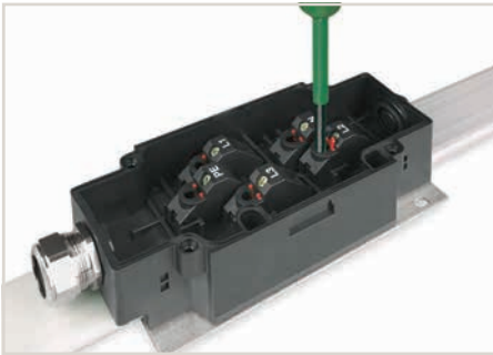
Red contact clips confirm that the contacts are made correctly when they are flush with the terminals.
