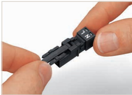
All connectors for fixed installations (snap-in versions, pluggable PCB connectors, distribution connectors) are factory-equipped with locking levers to ensure plugs and sockets are securely locked. Additional locking levers are only required for "flying leads" (plug/socket).
