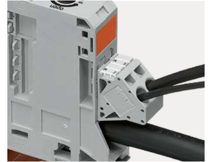
Power tap provides safe and easy power distribution to additional loads. The tap is inserted when the spring is retracted (for 50 ... 185 mm 2 high-current rail-mounted terminal blocks).
