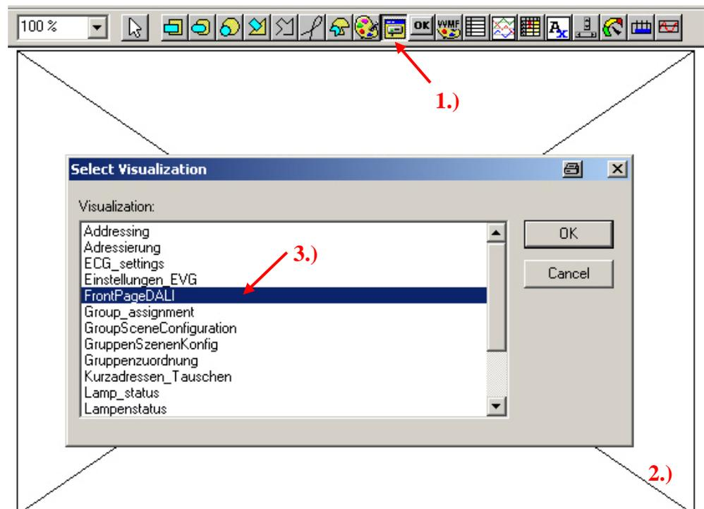
Figure 3: Calling-up the DALI configuration interface
