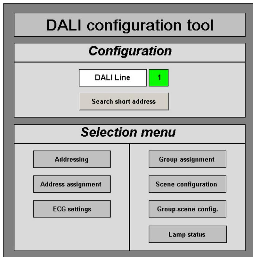
Figure 5: Front page of the DALI configuration tool.
