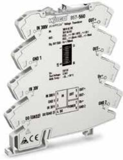
JUMPFLEX® Voltage Signal Conditioner; current input signal for AC and DC voltages; current and voltage output signal; digital output; configuration via software/DIP switch; 24 VDC supply voltage; 6 mm wide
