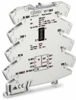
JUMPFLEX® Power Signal Conditioner; current and voltage input signal; current and voltage output signal; digital output; configuration via software/DIP switch; 24 VDC supply voltage; 6 mm wide
