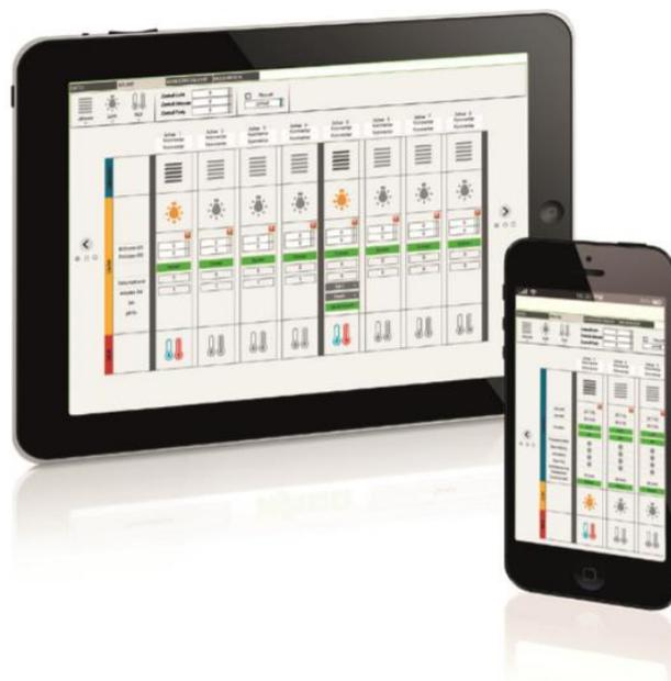
In the new version of **flexROOM®** the graphic user interface for configuration can be called up on smartphones and tablets. Users can modify all individual settings and view the system status.
