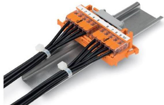
Four different mounting options are possible with the new mounting carrier. The simplest method is snapping the carrier vertically onto the DIN-rail, or, as shown here, mounting it horizontally on the DIN-rail using a 222 Series Angled DIN-Rail Adapter (222-510). The carrier can also be screwed to smooth, flat surfaces if necessary.
